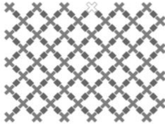
Figure 1. Connection-scheme of a 53 (working)-qubit Sycamore processor (adapted from Arute et al. 2019a, 505). Solid crosses denote qubits that work; outlined crosses denote qubits that don't work.
