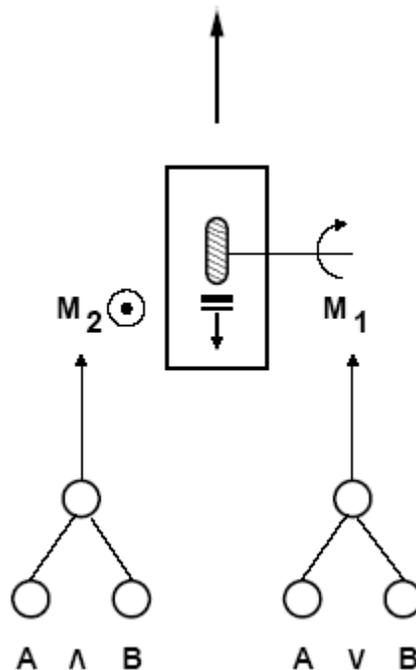
Figure 2: The XOR Robot. This robot has one wheel, with two actuated degrees of freedom. The motor M1 is responsible for turning the wheel so that the robot moves forward. The motor M2 is responsible for lifting the wheel off the ground. Each motor is controlled by a separate perceptron network, which takes as inputs A and B. M1 is controlled by a network which computes A OR B, and M2 by a network which computes A AND B.
