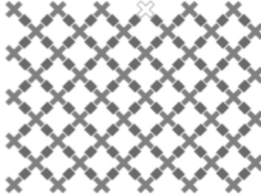
Figure 1. Connection-scheme of a 53 (working)-qubit Sycamore processor. Solid crosses denote qubits that work; outlined crosses denote qubits that don't work. "Squares" represent "adjustable couplers" (adapted from Arute et al. 2019a, 505).
